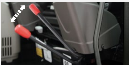
Safety lever to access the cockpit
