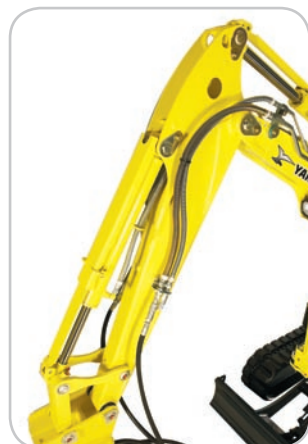
> Extension of the 3 rd circuit.
