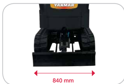
Extended undercarriage for better stability
