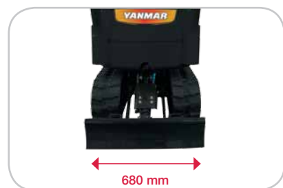
Retracted undercarriage to allow easier manoeuvre
