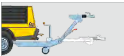
Height-adjustable towing hitch with run-on and parking brake
