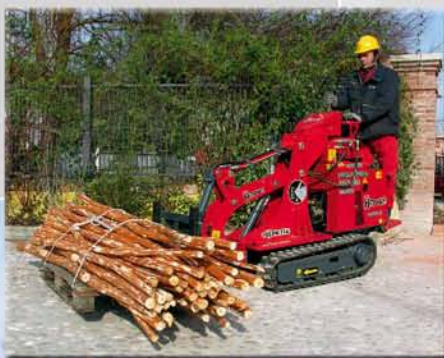
KIT RHINETTA CON PORTA PALLETS KIT RHINETTA WITH PALLETS FORKLIFT
