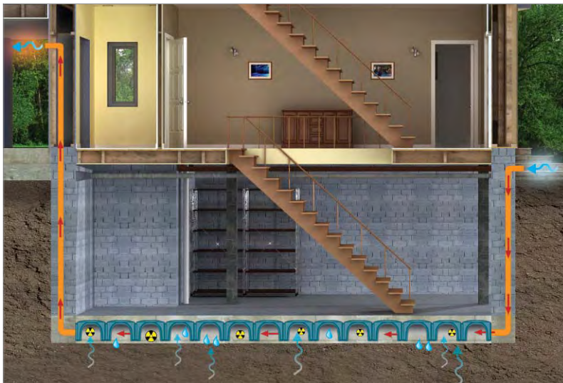
Home built with a ventilated IGLU® foundation.
