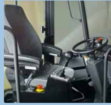
Integrated cockpit with rotating seat
