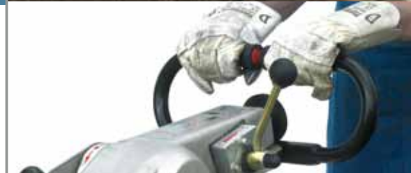
Dead man's handle with electronic sensors (Optional)
