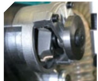
Separate copier from the bit.
