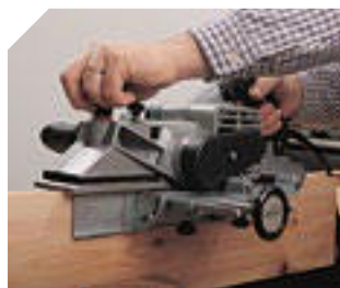
Micrometric fence. For making bevelled edges at different angles.
