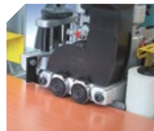
Simultaneous top and bottom trimming, with radius or 10^\circ chanfer. Flat scrappers after the trimming unit.
