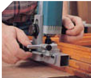
Slotting a window, flashing side.
