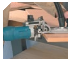
Trimming the edge with the straight bit.
