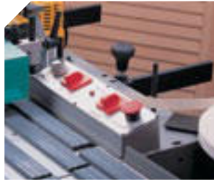
Safety control (STOP). Electronic temperature control.
