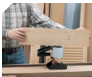
Gluing with the upper roller.
