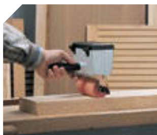
Gluing with vinyl (white) glues
