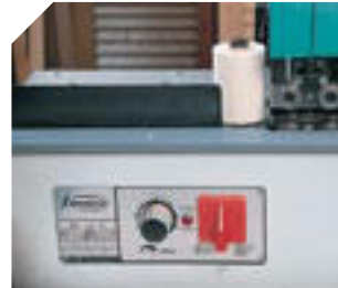
Electronic temperature regulation.
