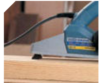
Rest shoe to avoid the blades touch and damage the surfaces.
