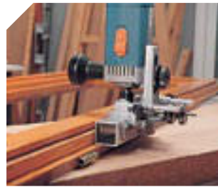
Slotting a window, hinges side.
