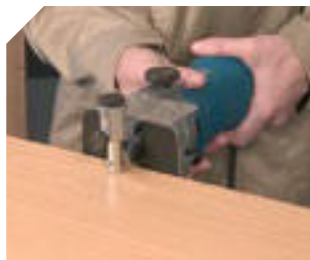
Excellent finishing when trimming laminates.
