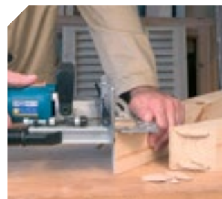
Stronger joints with No. 6 splines.
