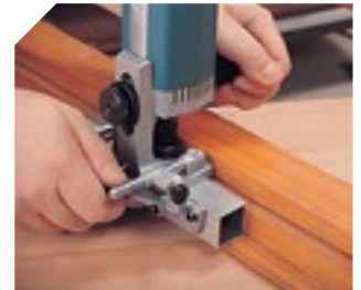
Slotting a window, lock side.
