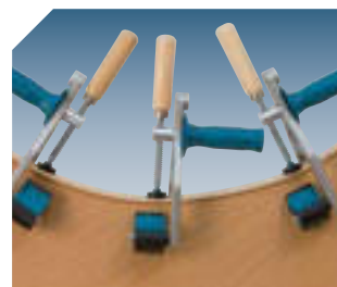
Fixing tapes on concave panels
