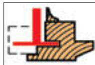
Slotting a window, flashing side.
