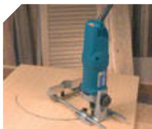
Trimming circular slots.
