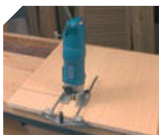
Trimming parallel slots.
