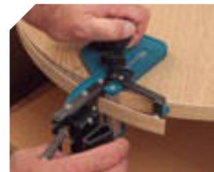
Cutting on circular panels.
