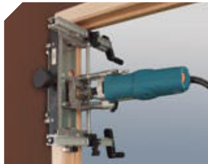
Making the upper recess on the frame.
