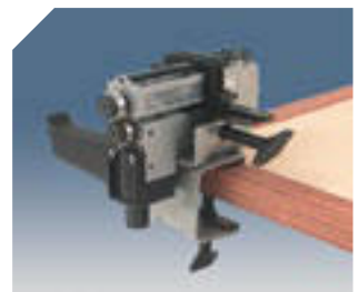
TK78 stand for securing to a workbench.
