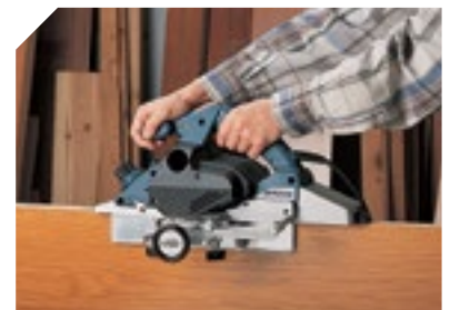
Micrometric fence for making bevelled edges at different angles.
