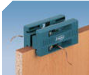
Trims both sides simultaneously.
