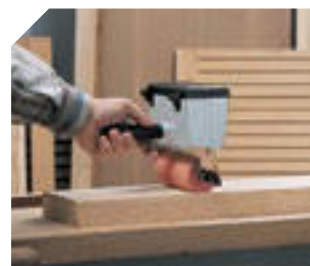
Gluing with vinyl (white) glues
