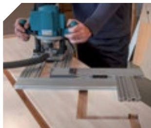
Quick and easy routing of the recesses on the stringers
