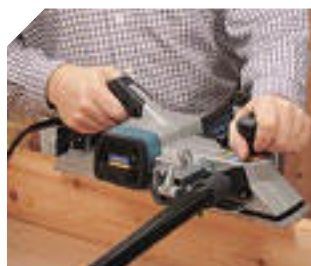
Dust collector connection.
