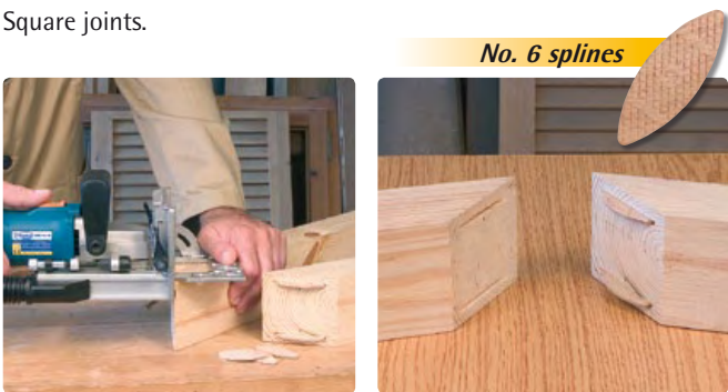
Stronger joints with No. 6 splines.
