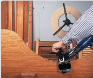
Possibility to band straight, circular or shaped pieces.
