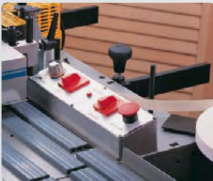
Safety control (STOP). Electronic temperature control.
