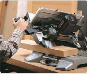
Base is one block giving a large supporting area. A new table with nongrip turning system.
