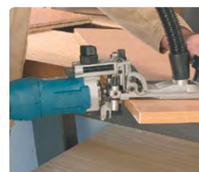
Trimming the edge with the straight bit.
