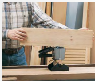
Gluing with the upper roller.
