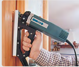
With centering pivot easing entry of the bit at the start of slotting process.
