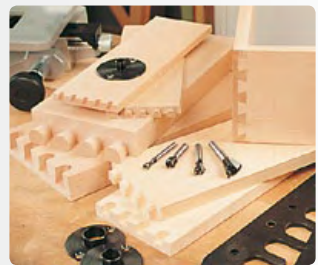
4 types of dovetail joints. Perfect finish on dovetail joints.
