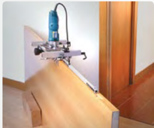
To make other recesses both on frames and doors it is not necessary to readjust the machine.
