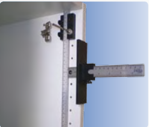
Drilling for placing invisible hinges.
