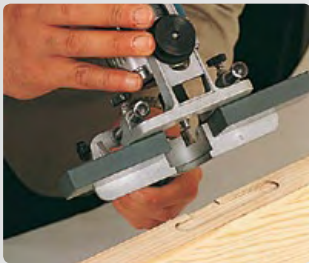
Placing hinges with the ZB93 head.
