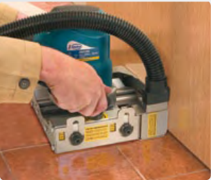
Its cutting depth allows it to cut the doors at once without splintering.
