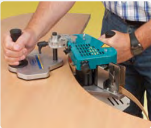
Perfect clamping for working with the PEB250 edge banders.
