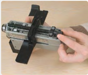
Micrometric regulation of the cutting width.
