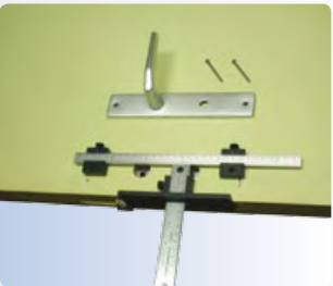
Drilling for door accessories.
