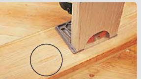
Stronger joints with No. 6 splines.
