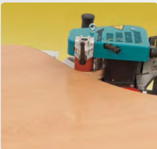
Easy banding of shaped and round panels.
