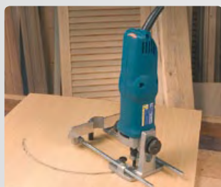
Trimming circular slots.
