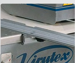
Easy adjustment of the cutting wide.
