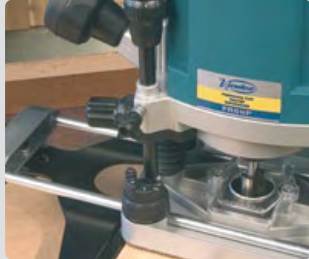
Six adjustable depth positions for rapid selection of the desired routing depth.
