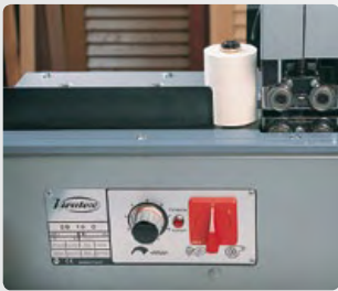
Electronic temperature regulation.
