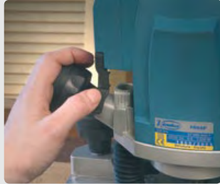
On-Off switch and head blocking may be activated from the knob, giving total, safe control of the machine.
