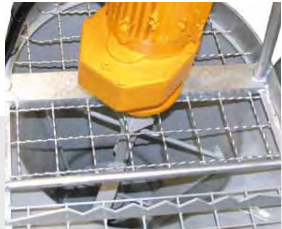
The large Sprayboy hopper, in which you mix the material before it is pumped.
