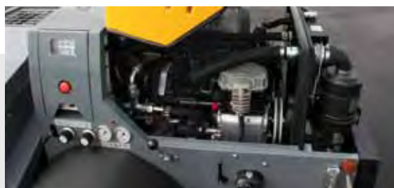
The maximum motor speed of just 2,400 rpm and the good sound insulation make the SP 11 into a machine that is quieter than average.
