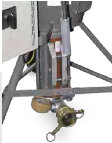
Discharge connection with pressure gauge for connection of the mortar hoses.
