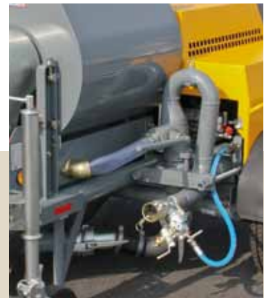
The pressure connection of piston pump KA 230 in the P 13 for the hose connection
