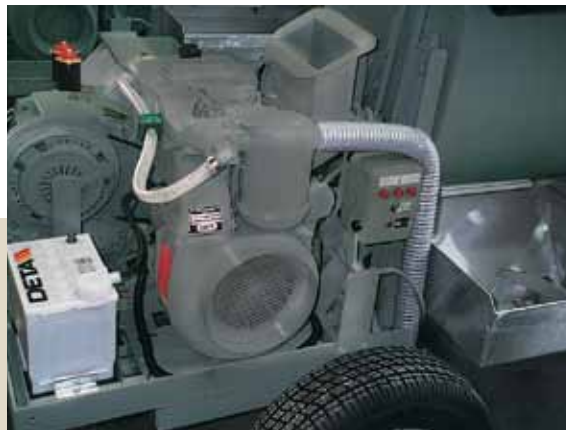
The powerful 2-cylinder diesel motor works in a relatively low speed range and is extremely robust and requires low maintenance.
