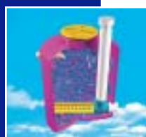
AEROBIC TRICKLING FILTER BASED PLANTS
