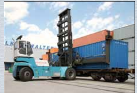
container - rail loading
