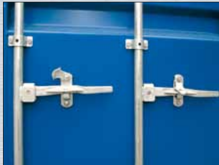
forged and galvanised door locking bars
